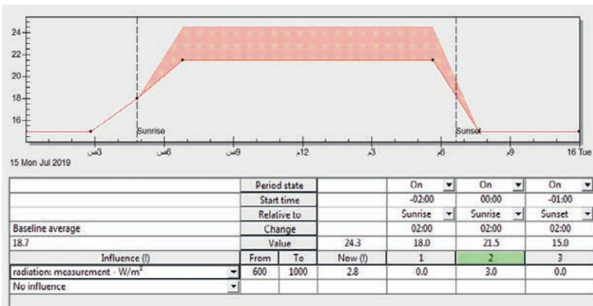
**Figure 19** If more radiation, from 600 to 1000 W/m<sup>2</sup>, ventilation starts at a 3°C higher temperature.
