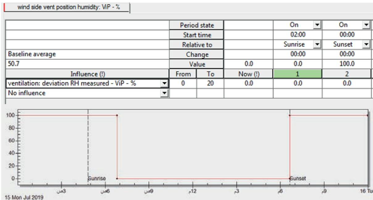
**Figure 20** If RH measured is 0-20% higher than the setpoint, the windows will gradually open. More than 20% difference will open the windows completely.
