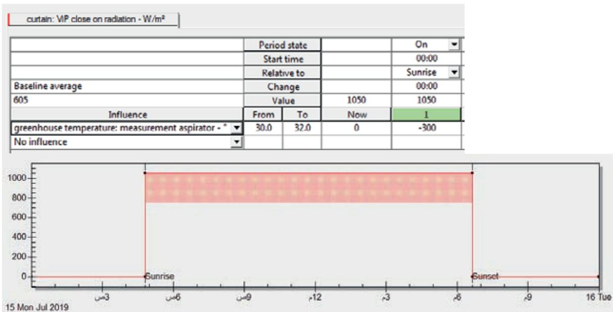
**Figure 21** Shading at high radiation and high temperature.
